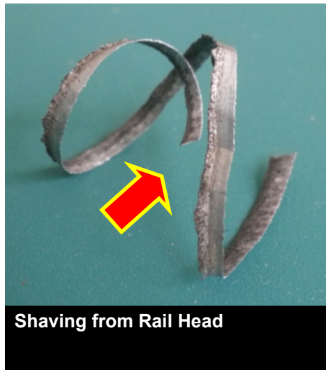
Damage to Switch Point
