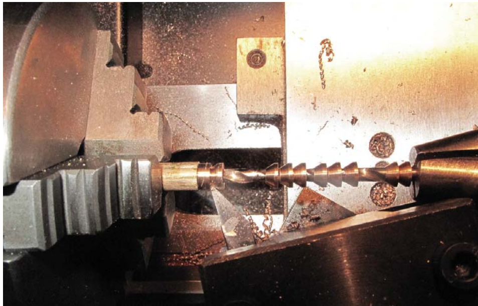
Fig.3. Setup for making union cones as tool nears end of cut. Note slight angle between tool's right cutting edge and surface of cone. Previously made cones are stacked up on drill to save time in production.
