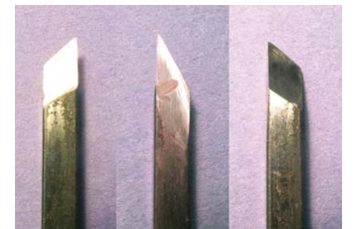
Fig.2. An LBSC dual-function lathe tool, showing ground and stoned surfaces on left side, top and right side.
