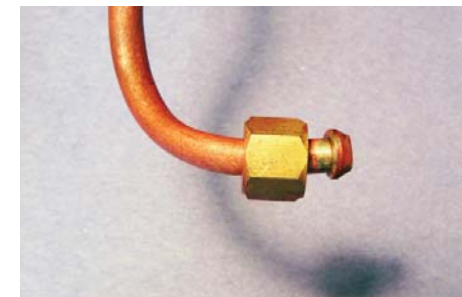
Fig.5. Completed nut and cone on end of a \frac{1}{8} " pipe
