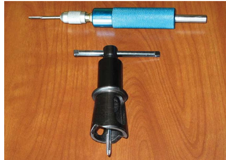
Photo 2. (Top) Tap holder for use in a lathe. (Bottom) Tap for right angle cuts.
